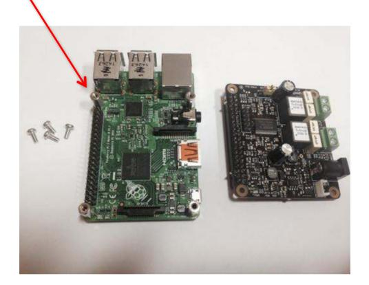
Once the Pi-DigiAMP+ has been fitted the remaining screws can be tightened (finger tight please) as
