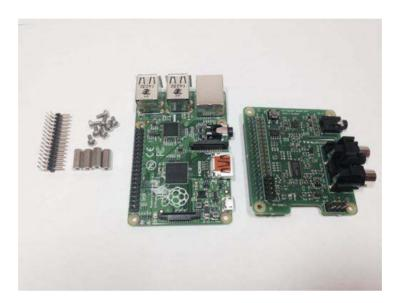
The spacers should be screwed (finger tight only) to the Raspberry Pi before adding the Pi-DAC+.
