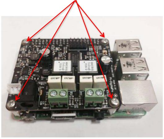
If you are using the Pi-CASE+ then replace the 4x screws beneath the Pi with the 4x 5mm PCB standoffs provided with the Pi-CASE+
